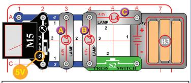
Part A: Set the meter (M5) to the 5V setting. Push the press switch (S2) for several seconds, while watching the meter. The meter is measuring the voltage across the two left lamps (labeled A & B); its reading jumps up when the switch is pressed, then slowly rises more for a few seconds. Push the switch again while closely watching the lamps A & B. Notice how lamps A & B initially are off, but turn on dimly within a second or two.
