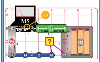
Build the circuit shown; the anything you want. Set the meter (M5) to the 1A setting and turn on the switch (S1). Touch various materials between the snaps on the 4-snap wire and battlery holder "—" side. Use the red jumper wire to help make a connection if needed. See which materials are good at transporting electricity by watching the meter current and lamp (L4) brightness.
