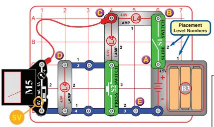
The circuit has three lamps connected in series, or two when S2 is pressed (S2 bypasses the last one)
