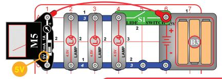
Set the meter (M5) to the 5V setting, and initially keep the switch (S1) off. The meter measures the battery voltage with the lamps (L4) off.
