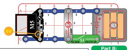
Set the meter (M5) to the 5V setting, and turn on the slide switch (S1). The lamp (L4) comes on, and the meter measures the voltage from the 3 batteries.
