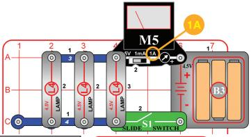
Modify the preceding circuit to match this one. Set the meter (M5) to the 1A setting and turn on the switch (S1). The meter measures the current. Try removing one or two lamps and see how the current changes. Also try this circuit with both new strong batteries and with old weak ones.
