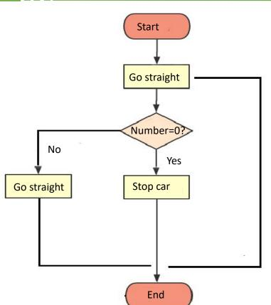
The numerical value that both the line tracking sensors (fitted on left and right sides) will return is 0 after the detection of the end line, so when the receiver tubes of sensors return 0, the bot should immediately be stopped. Though, in sprint phase the Q scout returns 3.
